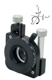
This kinematic mount accepts crystal housings of Ø25.4 mm and thickness up to 10.5 mm. The housing is stopped by a rest-flange inside the central aperture of the platform, and is secured by a threaded retaining ring.
